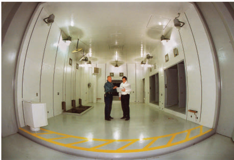
The largest of the Gamma Irradiation Facility's three test cells at Sandia National Laboratories is spacious enough to irradiate large objects like tanks and satellites.
